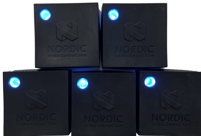
Figure 4.3 First mesh network, using multiple Thingy:52
